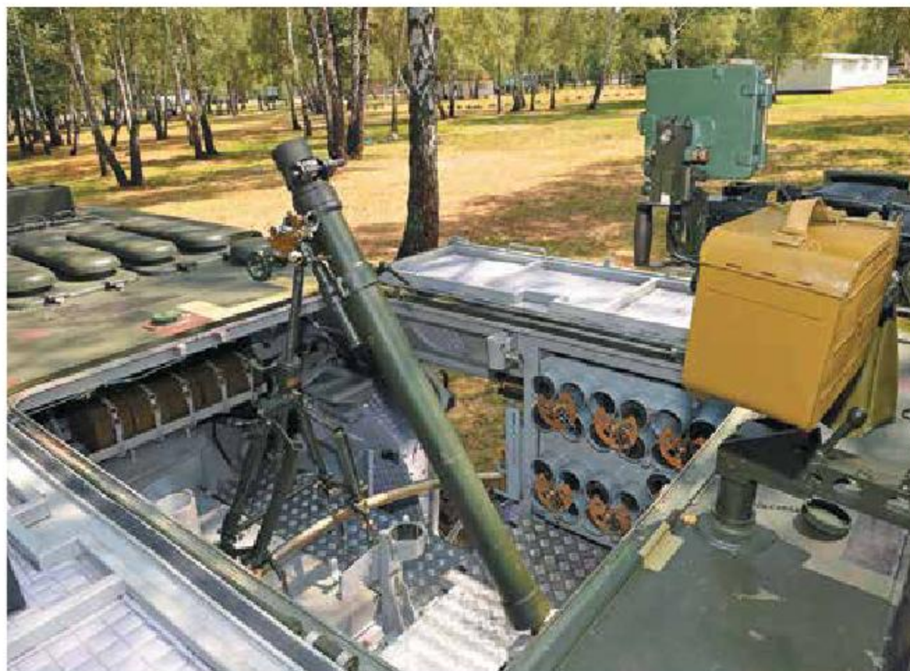
Kiev Armor Plant developed BTR-3M2 APC upgrade equipped with a 120-mm mortar and the 12.7-mm NSVT machine gun.
