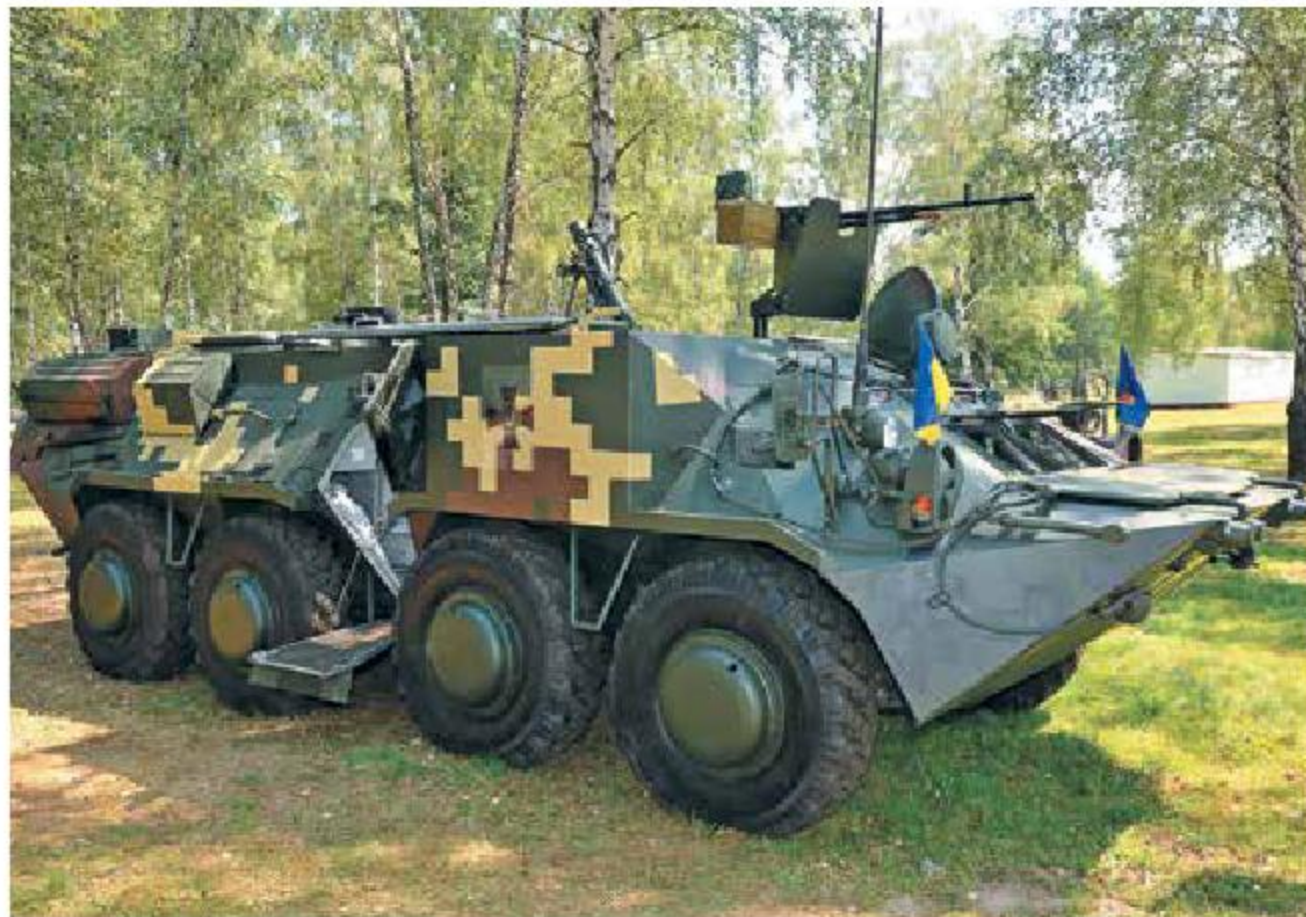
Kiev Armor Plant developed BTR-3M2 APC upgrade equipped with a 120-mm mortar and the 12.7-mm NSVT machine gun.
