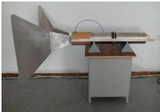
Prototype missile ammunition with deployed horn TEM antenna ready to install
