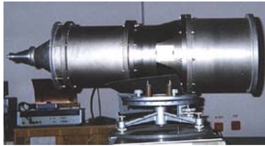
Combined coaxial-sector antenna and mode converter
