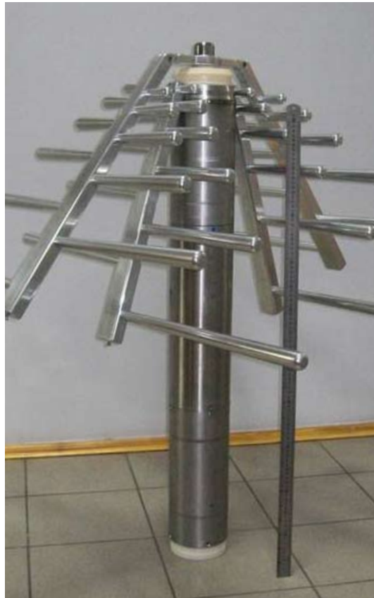
Prototype ammunition (electromagnetic bomb) with logo periodic antenna
