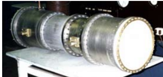
General view of MILO with combined mode converter and coaxial-sector antenna with output dielectric window
