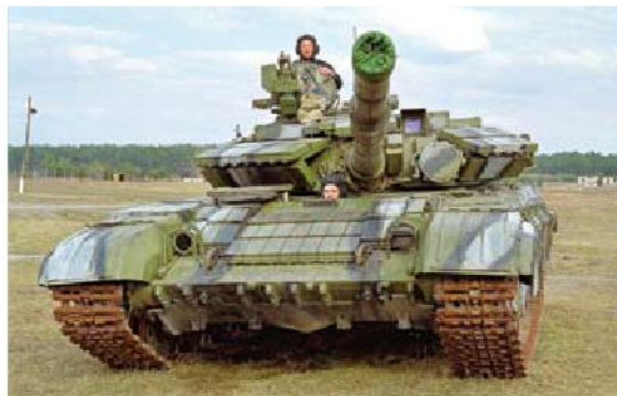
4 T-64BV-1, the overhauled configuration of the T-64 tank. The overhauled T-64BV-1 is available at an average price of $200-250,000 per unit
