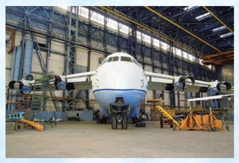
rainian-Russian power package integrating Motor-Sich D-27 engines with Aerosila SV-27 propfans, respectively. This combination allows for high cruising speeds, simultaneously reducing fuel consumption by 20-30 percent compared to current-generation turbojet counterparts.
