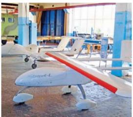
The tactical UAS 'STREPET-L' has a maximum take-off mass of 80 kg, including a 20kg pay-load. Effective range is put at 80 km and practical ceiling at 4,000m. Fuel endurance is enough for up to four hours in the air at a cruising speed of 130 kph.
