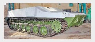
Kharkiv Armor Repair Plant has developed and built a new armored fighting platform that shares power plant and related servicing systems as well as transmission, chassis and electric equipment with the T-80 main battle tank and Oplot tank, Ukraine Industrial website reported on April 17, 2013. The platform is powered by a 6TD-2E engine developing 1200 hp, and provides high-level basic protection. In the armored personnel carrier configuration, the troop compartment is equipped
